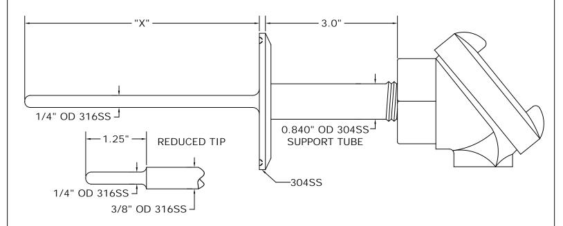
Clean in place (CIP) style sanitary connected Thermocouples are used in the bevarage, chemical, dairy, food and pharmaceutical processing industries. Acrolab offers the most common sanitary caps in the industry and all meet 3-A Sanitary Standard 74-. The sheaths are 316SS and come with a FDA compliant white thermoplastic head. The assemblies provide excellent washdown protection. Reduced tips are offered for faster responce time.
